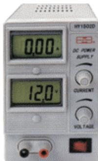
Two 3-1/2 digit LCD Display, accuracy: Voltage +/- 1% + 2 digits, Current: +/- 1.5% + 2 digits
